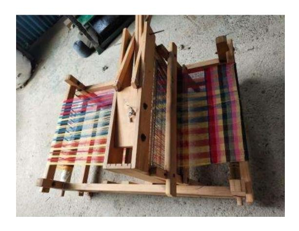
In order to Solve the problem of disabled weavers who cannot operate shafts by their legs, the innovators made a new mechanism by adding hand-levers to raise and lower the head shafts.
